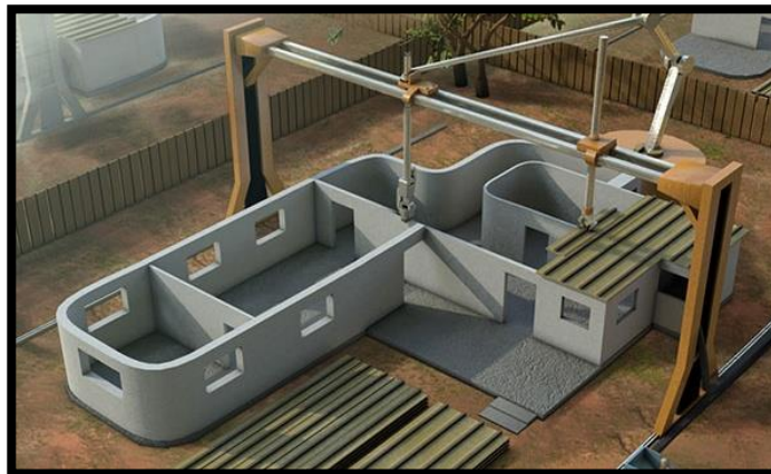
Figure 3: Large scale 3D printing - 'prints' quick-setting concrete from a computer controlled gantry.
