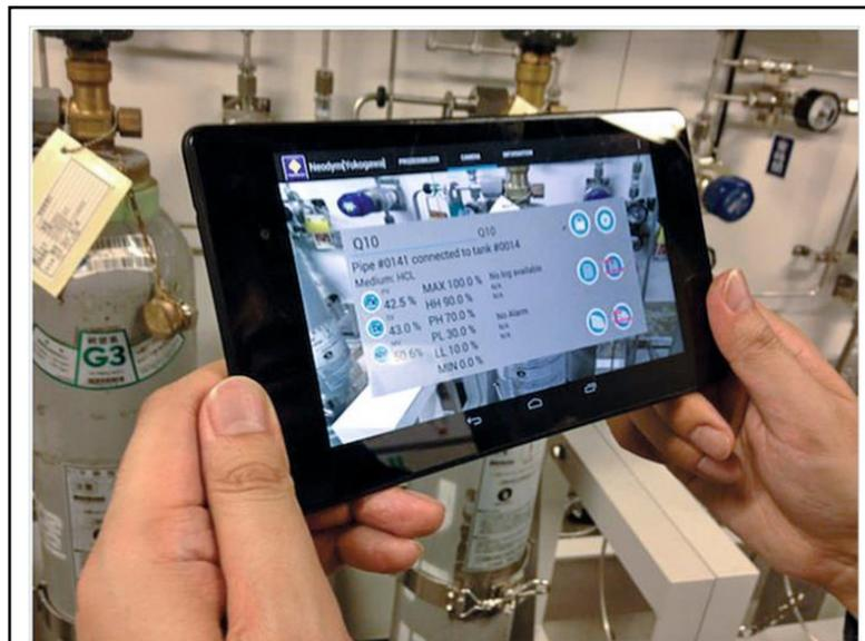
Yokogawa is a supplier of industrial automation systems. Working in collaboration with Akzo Nobel, the company has started field testing of the iMaintain augmented reality solution. iMaintain uses an Android tablet, which has a direct link to the process control system, to make information such as trend curves, alarms and operating instructions available to personnel working on site. (Picture: Akzo Nobel/Yokogawa)
