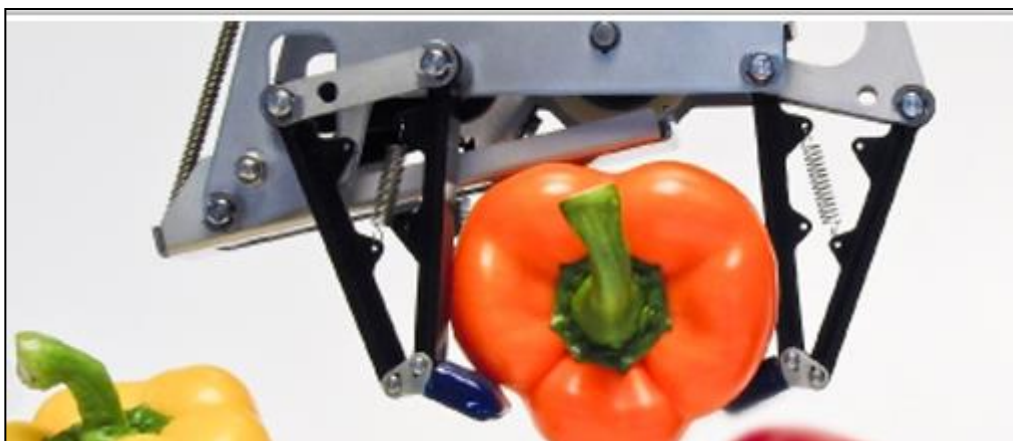
Figure 8: Lacquey's gripper Source: http://www.bobbierobotics.nl/partners
